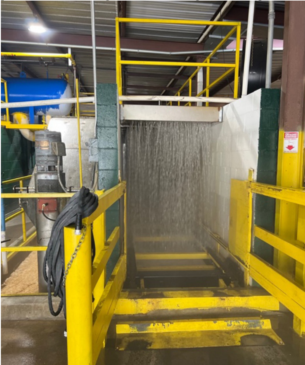
Figure 6. Hydrocooling System. With peaches, simply placing warm fruit in a cold storage room is not a very effective way of reducing temperature after harvest. A special method of field-heat
