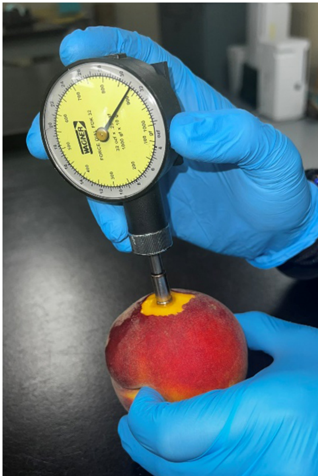
Figure 3. Firmness Measurement Using a Handheld Penetrometer. It is important to mention that the person measuring fruit firmness with these handheld penetrometers should place the fruit against a solid, immovable surface (like a tree trunk) to reduce measuring errors. To avoid sampling errors, measurements should be performed by the same person. A representative
