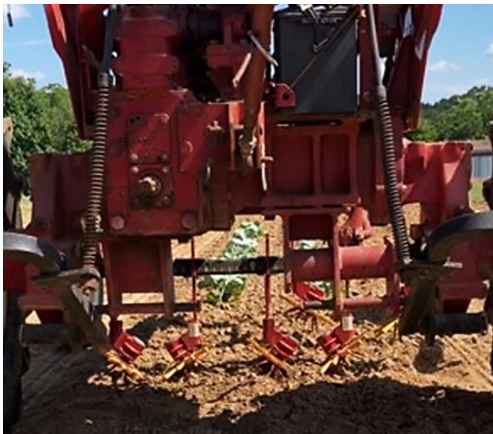
Figure 3. A tine weeder (left) and finger weeder (right) used in cultivation research. Drip irrigation lines are buried to a depth of roughly 4 in. so they do not interfere with cultivation and are not damaged by the equipment.
