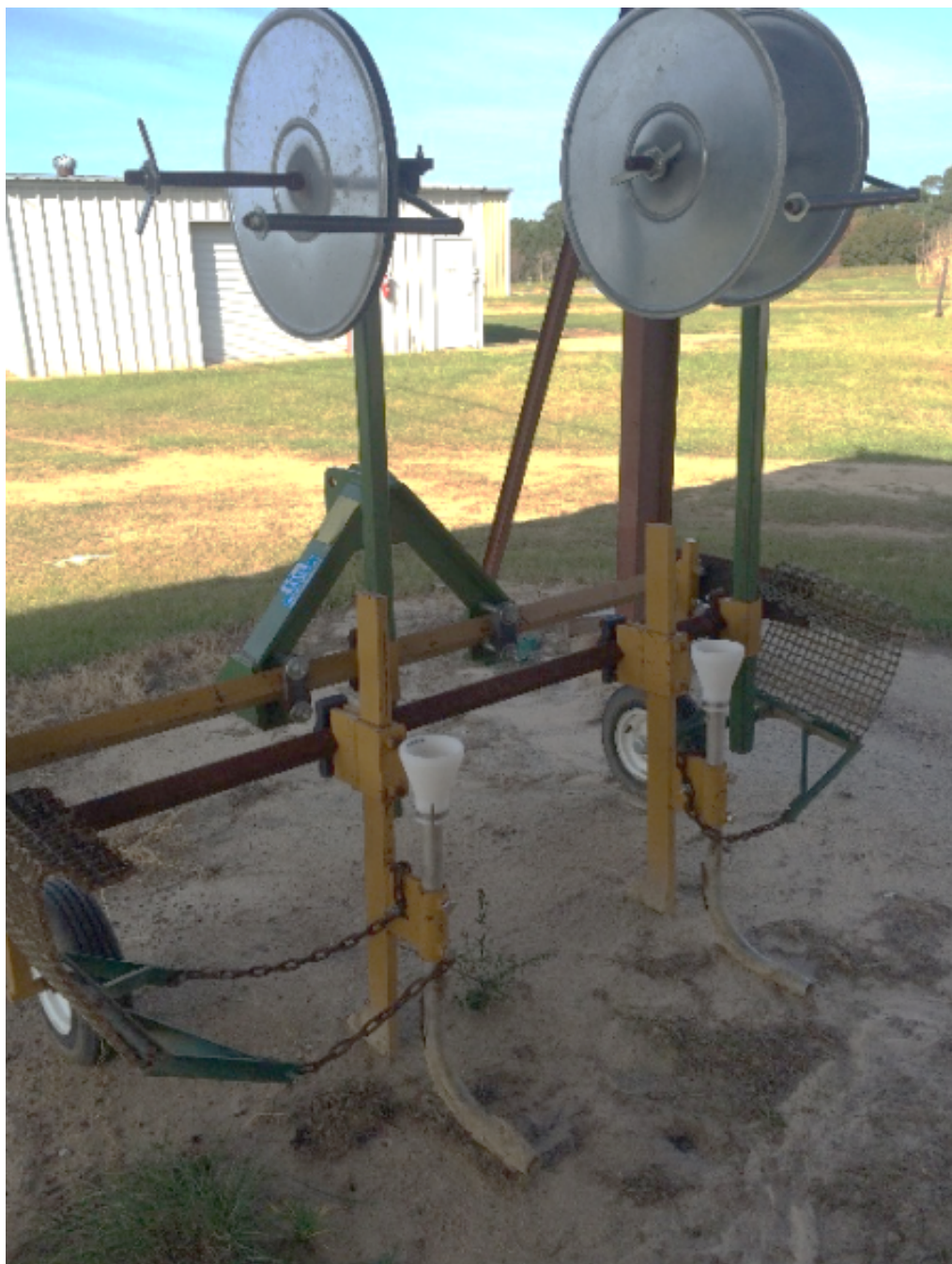
Figure 1. Two examples of SSDI tools. On the left is a sled-type device, while the implement on the right uses small tires to maintain a constant depth with the soil surface.
