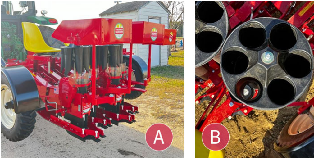
Figure 5. Carrousel-Type Transplanter With Four Transplanting Units (A) Versus a Single Carrousel (B).
