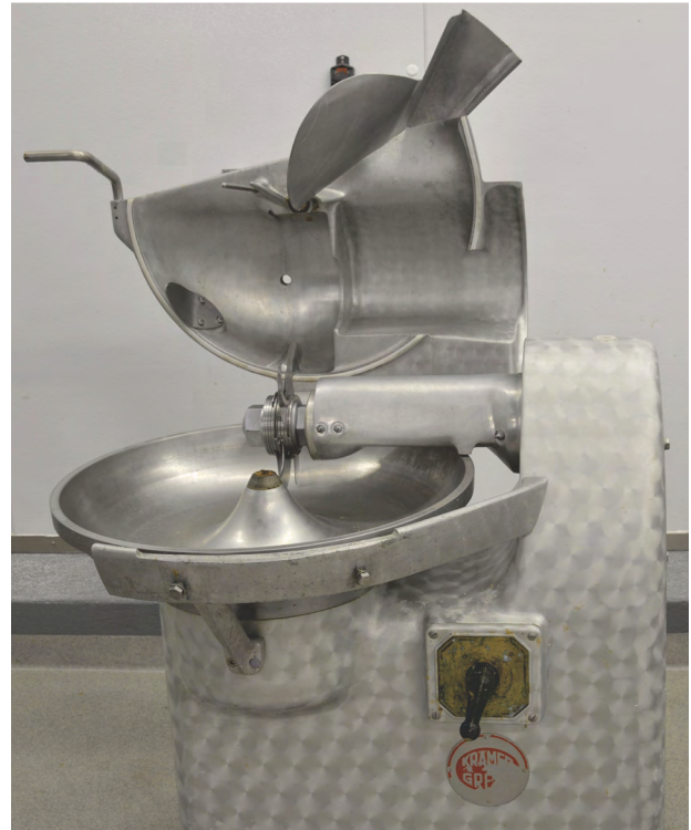
A bowl chopper is used to make a finely ground, emulsified sausage batter, as for bologna or hotdogs.
