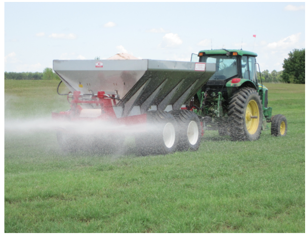
Figure 1. Example of a spinner-disc spreader application pass. This demonstrates the difficulty of determining pass-to-pass distance without skips or overlaps.
