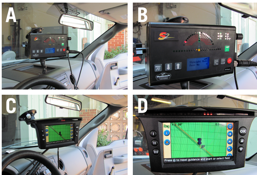
Figure 6. Examples of different types of lightbar guidance systems. A and B show the Outback Guidance system, which uses only lights to keep the driver on the line. C and D show the Trimble EZ-Guide, which has a row of lights at the top and an LCD display showing the guidance lines and current vehicle position in the field. As shown here, most manual steering aids can be used in any vehicle and are not limited to just tractors.
