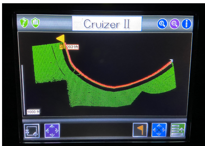
Figure 7. This device shows an area that was missed during alfalfa planting when using a lightbar guidance system. The area not covered is shown on the lightbar on the left, and this area in the field can easily be identified later in the season because the area was not planted.
