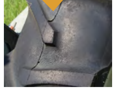
Figure 14. Cracks beginning to appear on tires. Cracks are typically due to weather wear and should be taken into consideration before the season starts. In some cases, system downtime costs more in yield than a single tire is worth.
