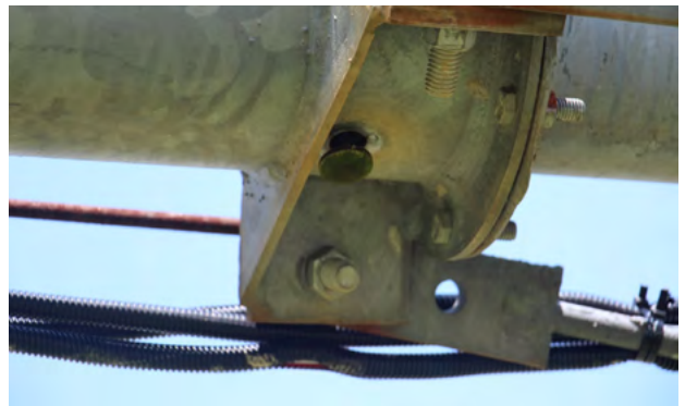
Figure 11. The drain valve for one of the pivot towers. In this case, the valve is open because there is no water in the system.
