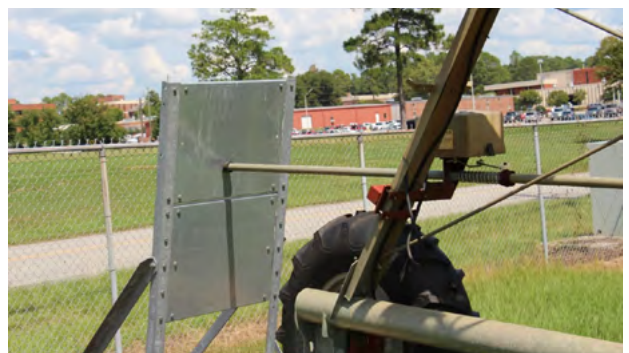
Figure 13. The stop and safety switch on a pivot. In this case, if either switch malfunctioned, the pivot would walk over the fence and into the road—a very dangerous situation.
