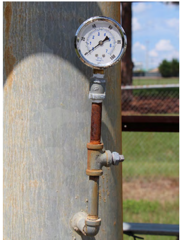
Figure 5. The main pressure gauge at the pivot point. The pressure should be the highest at this location and is an important position to verify proper pressure for pivot performance.
