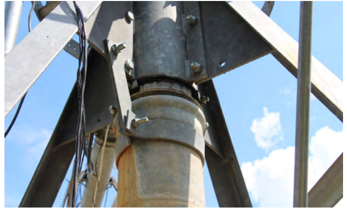
Figure 19. Visible signs of wear and use are often evident on the pivot point. In some cases, a closer inspection is needed. Carefully consider whether repair or replacement is needed.
