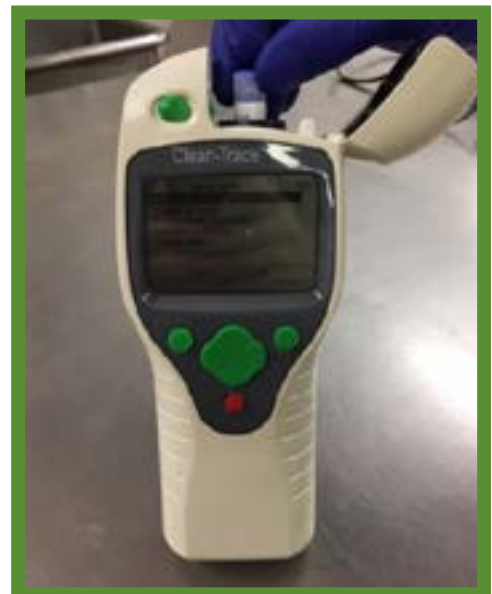
Figure 2. Placing an ATP swab in the luminometer for measurement.
