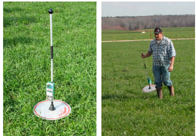
Figure 2. An electronic rising plate meter (left) can be used to measure pasture mass (right).
