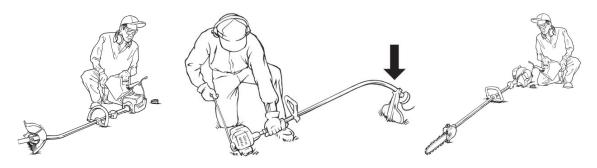
Turn off the motor and disconnect the spark plug wire before changing blades or doing any types of repairs or services. Rest equipment on ground when repairing or changing blades.
