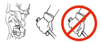
Fuel and start equipment on level ground. Use your arm, not your back, to pull the starter cord. When fueling equipment, never smoke, let equipment cool down before refueling, remove the fuel cap slowly and never over-fill the tank.
