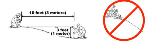
When mowing a slope with a push mower, start at the bottom of the hill and mow across the hill, from the bottom up to the top.
