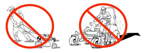
Never use a riding mower on slopes greater than 15° degrees or 27% slope. This is the almost the same as a drop of 3 ft. (1 m.) over a distance of 10 ft. (3 m.).
