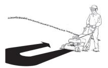
When mowing a slope with a riding mower, mow up and down the slope. Turn around on level ground at the top or bottom of the hill.
