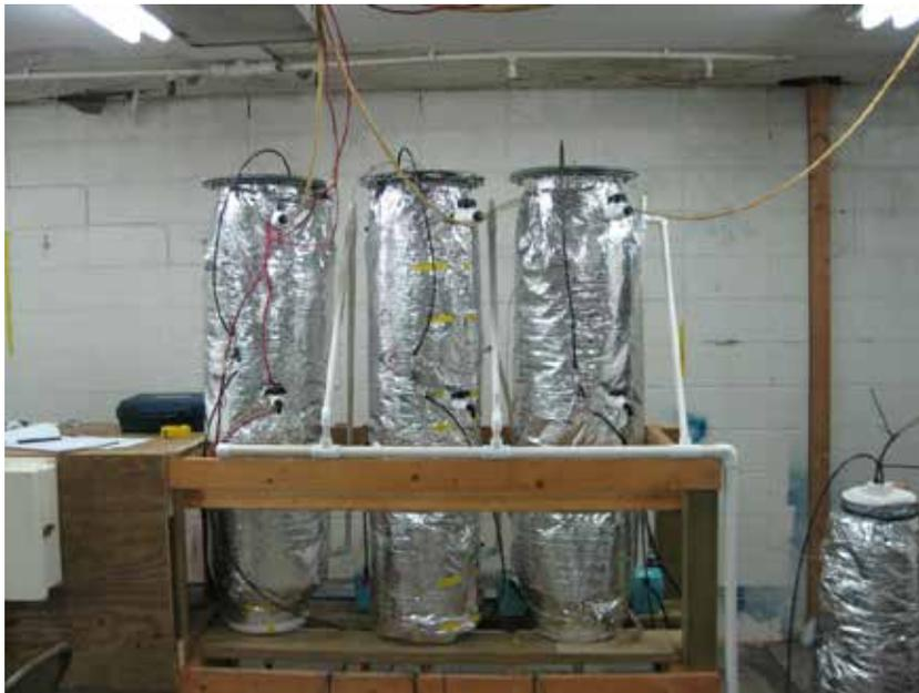
Figure 1. Anaerobic filters used in the experiments to determine amount of bio-gas that could be produced from onion culls.
