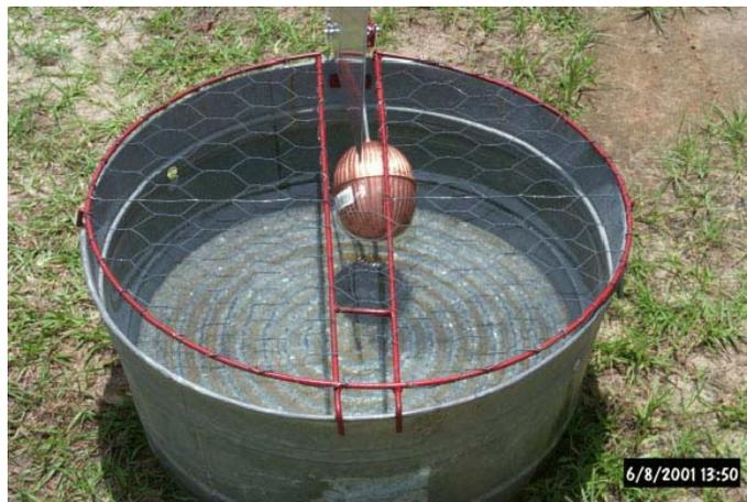
Figure 4. Basic covering screen with 2-inch mesh.
