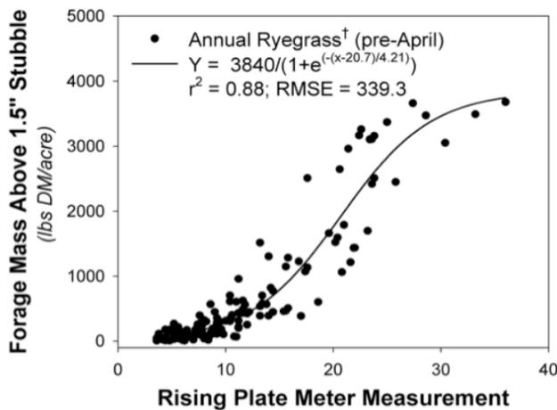
**Figure 4. The relationship between the rising plate meter measurement and forage mass above a 1.5-inch stubble height‡ for annual ryegrass prior to April 1. The equation represents the best fit for the data.**
