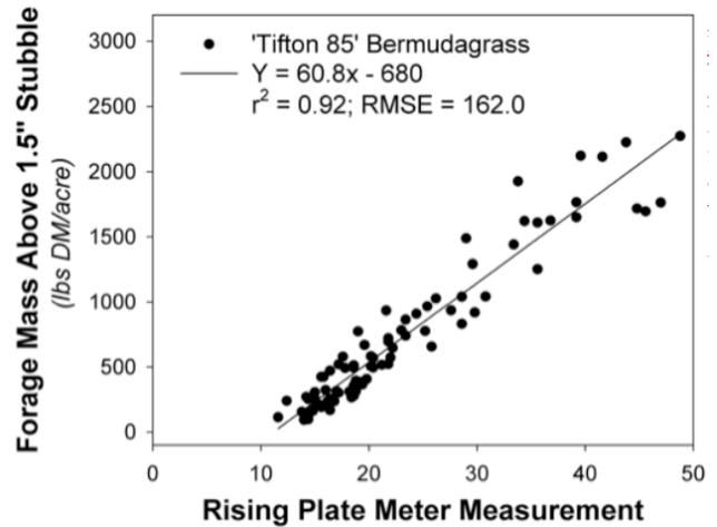
**Figure 9.** The relationship between the rising plate meter measurement and forage mass above a 1.5-in. stubble height† for 'Tifton 85' bermudagrass. The equation represents the best-fit for the data collected June through September 2010.
