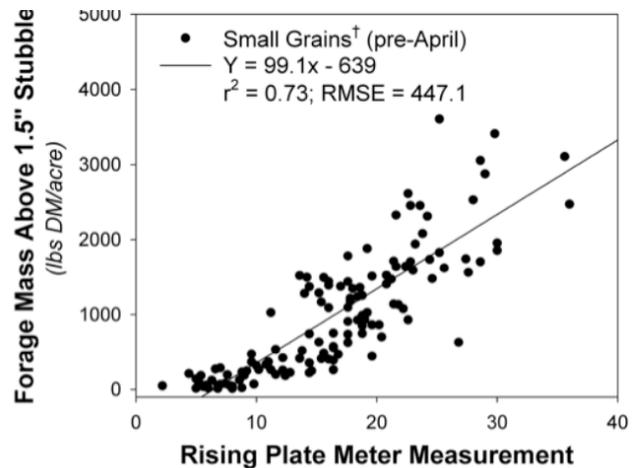
**Figure 5. The relationship between the rising plate meter measurement and forage mass above a 1.5-inch stubble height‡ for small grains prior to April 1. The equation represents the best fit for the data.**
