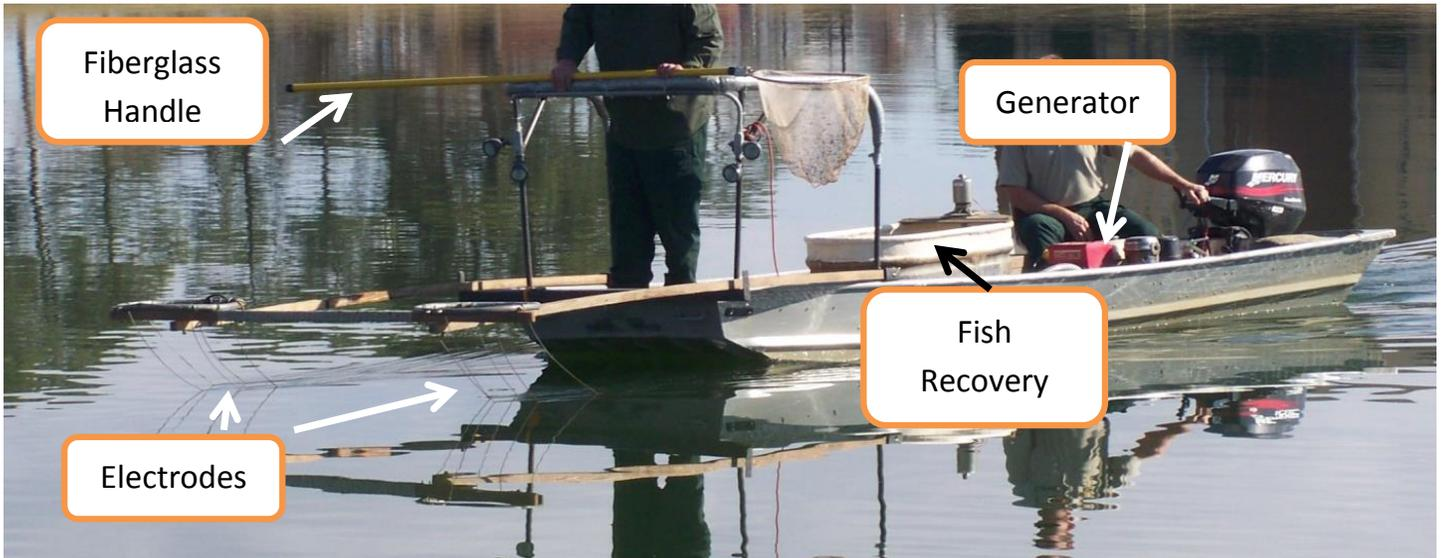
Figure 12. Electro-fishing equipment used to check pond balance or relocate fish.
