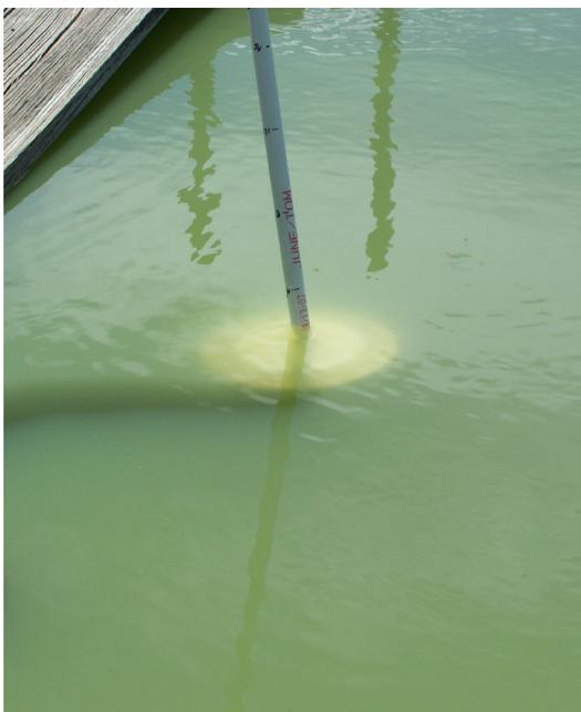
**Figure 6.** Using a white target on a stick to measure light penetration into pond water. The best range of light penetration is between 12 and 18 inches when using a pond fertilization program.
