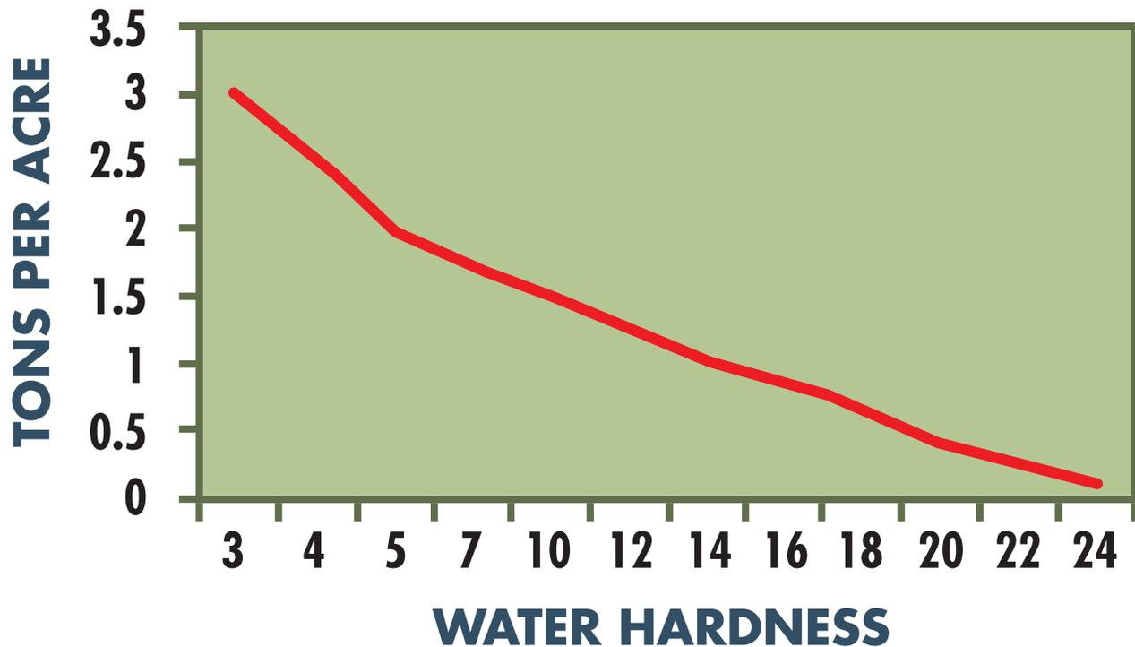
Figure 7. Lime required in ponds based on water hardness, showing little need for liming when hardness is above 20 ppm.
