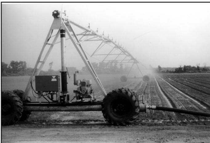
**Figure 6.** Hose-fed linear move irrigation system.
