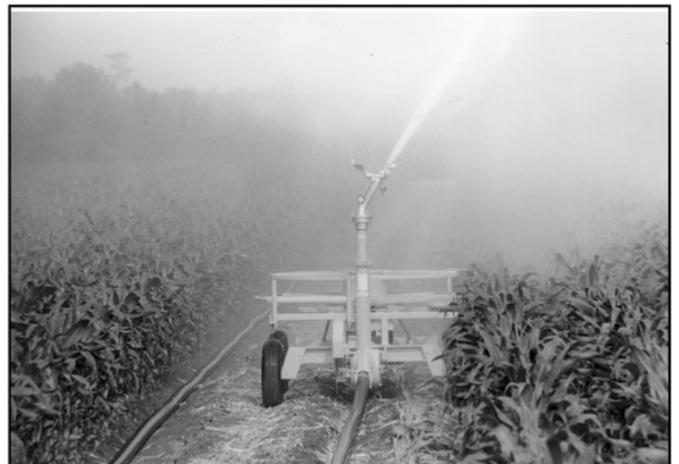
**Figure 7.** Cable-tow traveler irrigation.
