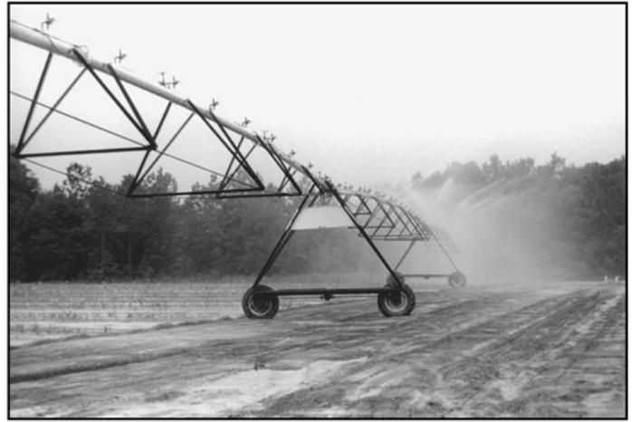
**Figure 3.** Center pivot irrigation system with medium pressure impact sprinklers.
