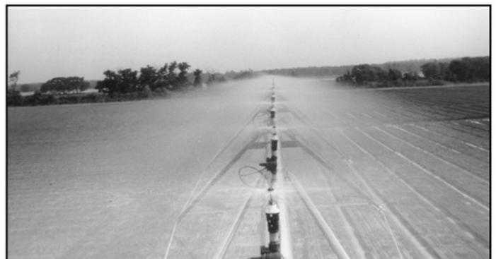
**Figure 2.** 360-degree spray nozzles with pressure regulators.
