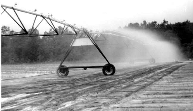
**Figure 1.** Center pivot irrigation system with low pressure spray nozzles.
