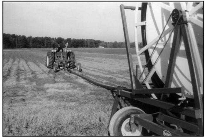
**Figure 8.** Hose-pull traveler irrigation system.
