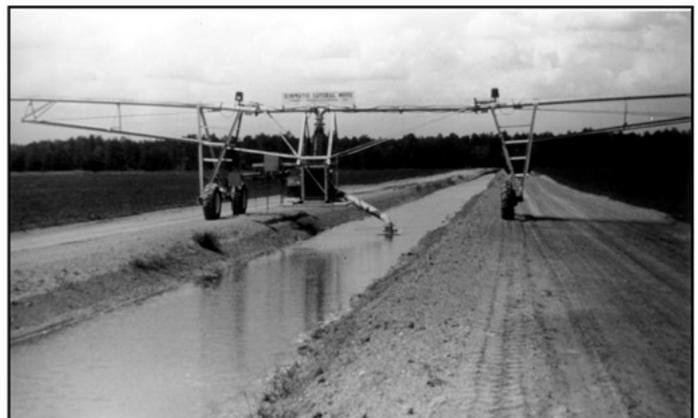
**Figure 5.** Ditch-fed linear move irrigation system.
