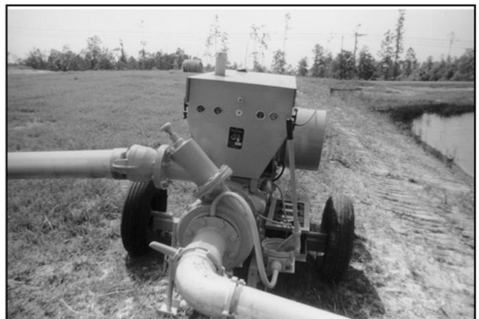
**Figure 15.** Diesel powered pumping unit on pond.
