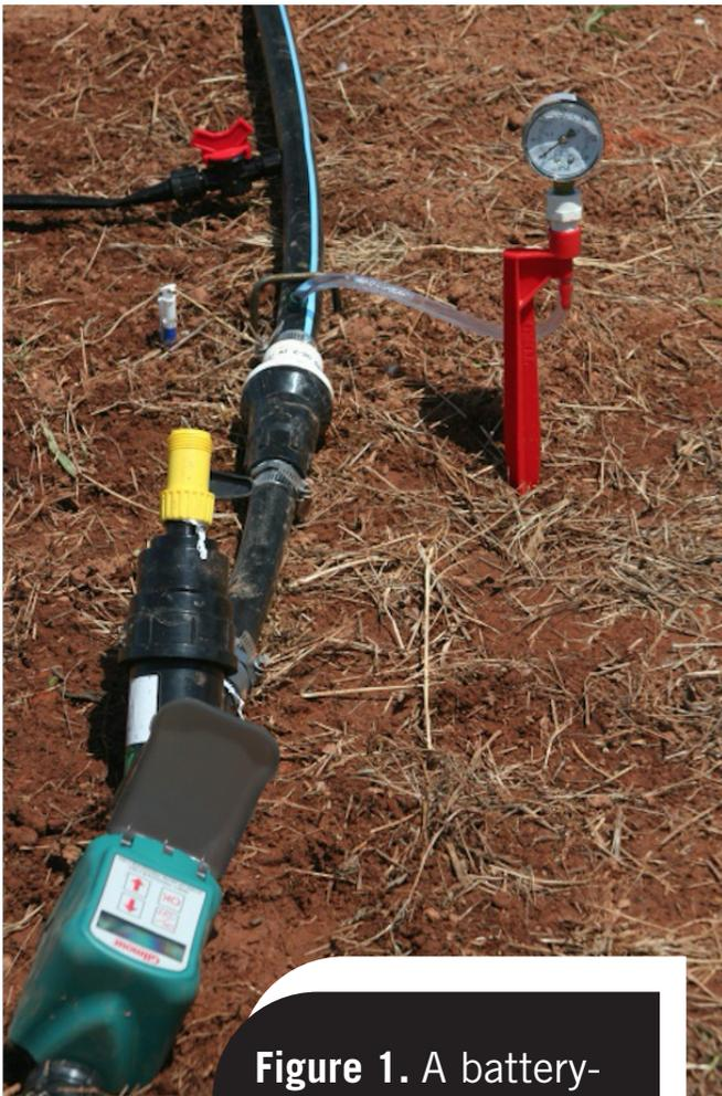
**Figure 1.** A battery-operated water timer helps to automate the drip irrigation system.
