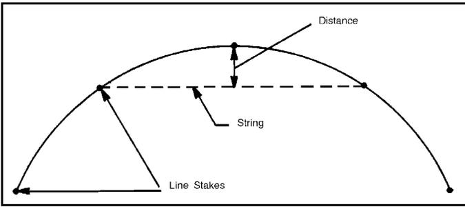
Figure 10. Fence post spacing around curves.
