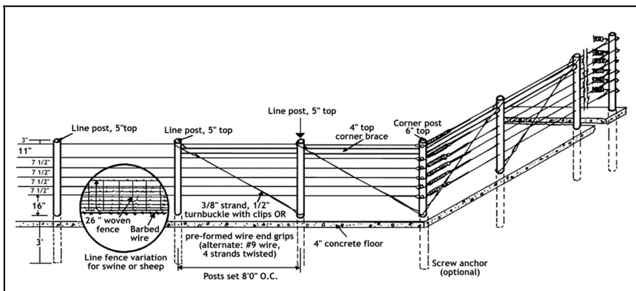
Figure 7. Cable fence — one type of installation.
