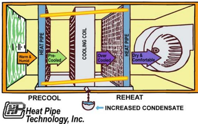
**Figure 2. Diagram of the heat-pump-dehumidifier. (Dinh, 1999)**
