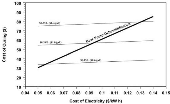
**Figure 12. Determining the break-even point for using either heat-pump-dehumidification or conventional curing according to the price of fuel.**
