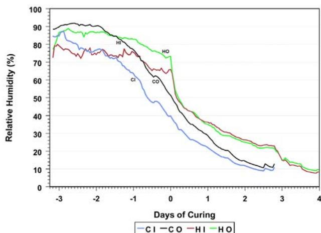
**Figure 7. Average relative humidity of supply and exhaust air for both conventional and heat-pump barns. CI = conventional in; CO = conventional out; HI = heat-pump in; HO = heat-pump out.**
