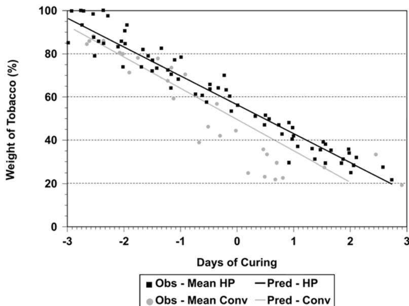
Figure 9. Regression lines representing the average rates of weight loss while curing in the heat-pump barn (HP) as compared with curing in the conventional barn (Conv).
