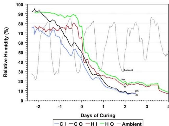
**Figure 8. Influence of the diurnal variation in ambient relative humidity throughout a cure upon the relative humidity of the supply and exhaust air for both conventional and heat-pump barns. CI = conventional in; CO = conventional out; HI - heat-pump in; HO = heat-pump out.**
