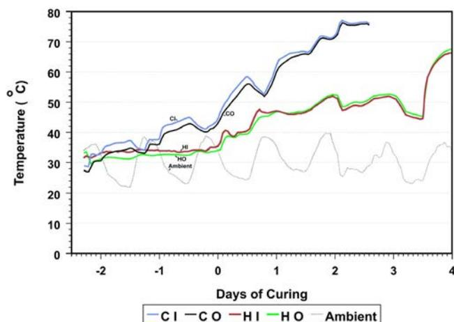
**Figure 6. Influence of the diurnal variation in ambient temperature throughout a cure upon the temperature of the supply and exhaust air for both conventional and heat-pump barns. CI = conventional in; CO = conventional out; HI = heat-pump in; HO = heat-pump out.**
