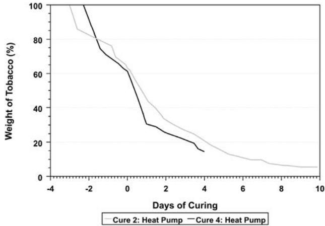
**Figure 10. Weight loss of tobacco both while drying with only dehumidification and drying with the assistance of high heat.**
