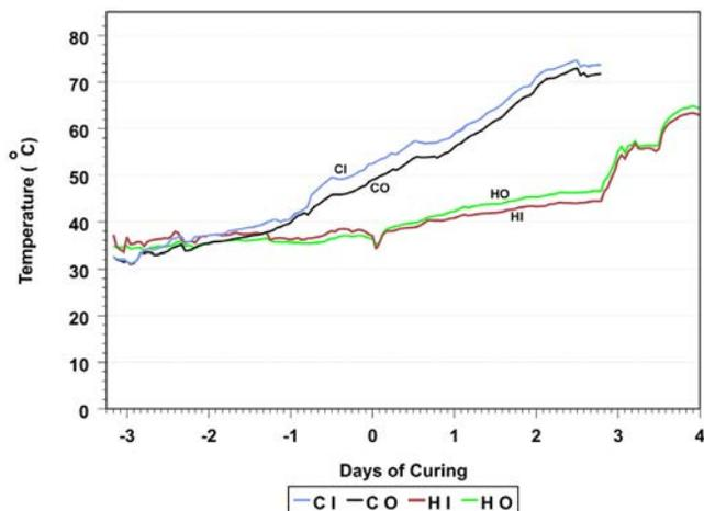
**Figure 5. Average temperature of supply and exhaust air for both conventional and heat-pump barns. CI = conventional in; CO = conventional out; HI = heat-pump in; HO = heat-pump out.**
