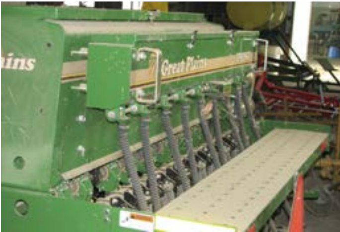
Figure 2. The no-till drill on the left has two hoppers so it can sow two cover crops at once (e.g., grass and a legume). In the photo on the right, note the coulters that are capable of opening a furrow.
