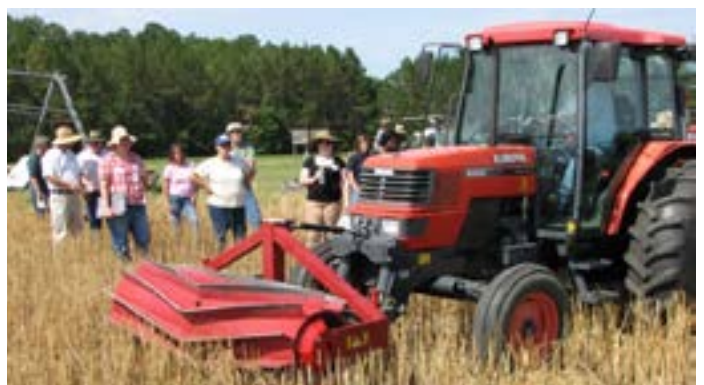
Figure 4. Roller-crimper mounted on the front of a tractor. Note the chevron design, which helps it ride more smoothly over the ground.
