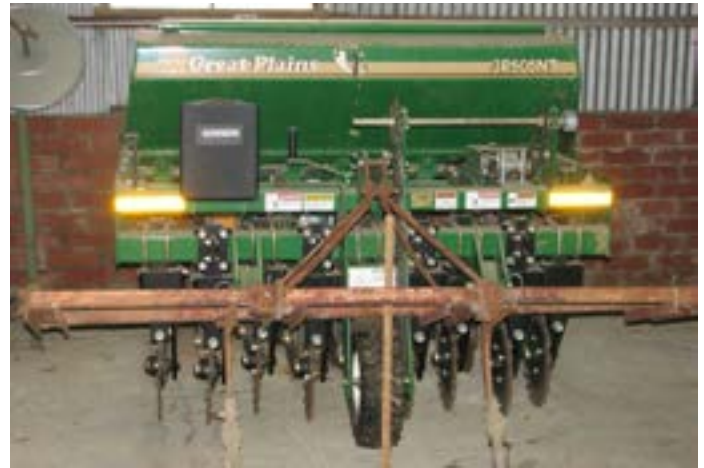
Figure 3. Single row no-till transplanter. Note this is a carousel-type transplanter.
